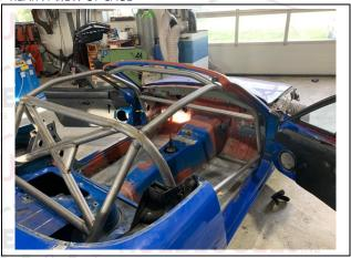
PHOTO 4 MAIN ROLLBAR TO FLOOR ATTACHMENT
